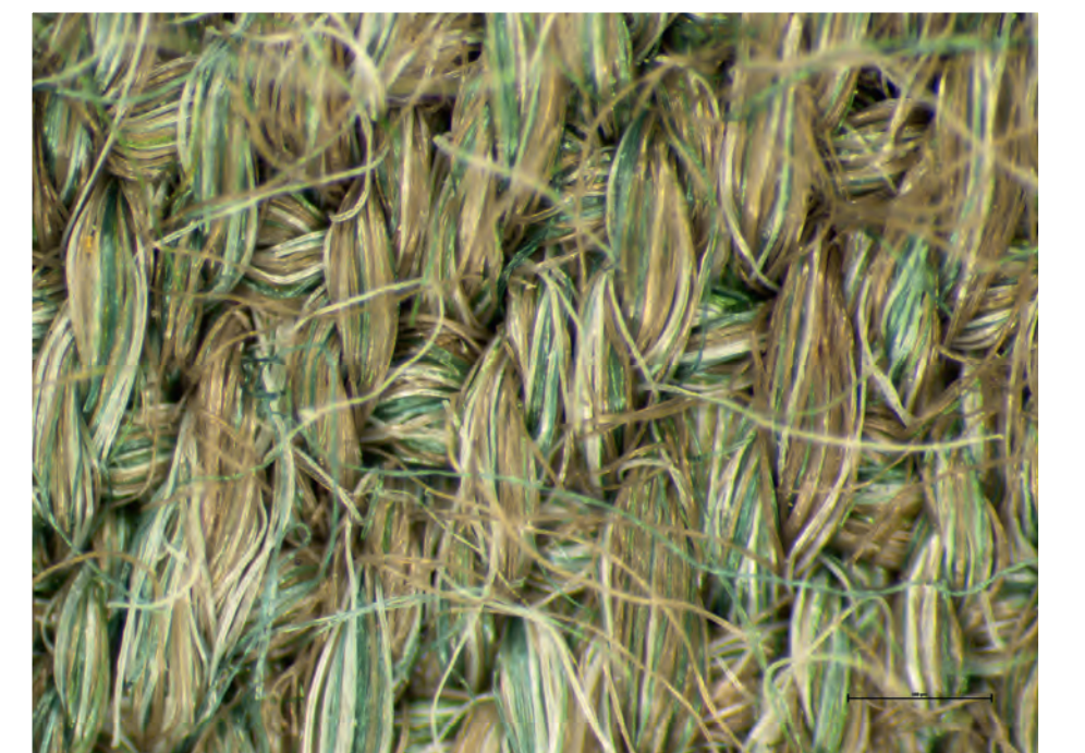
Base fabric at microscopic magnification 45x Photo Indra Saulesleja
